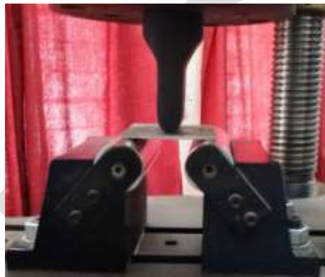
Fig 2. Test setup for three point bending.
