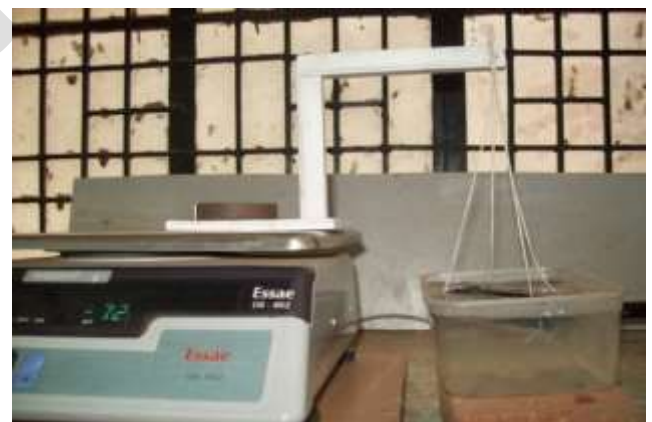
Figure 4.7 Sample weighed in distilled water
