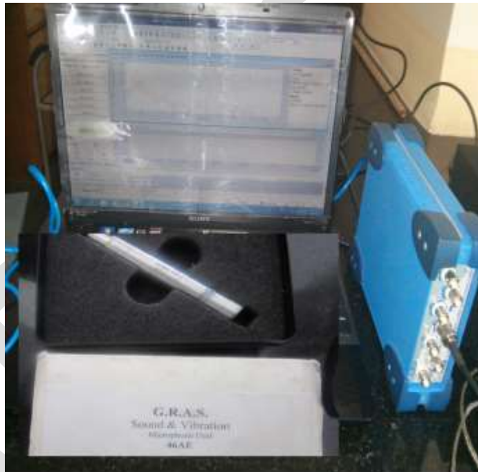
Figure 4: FFT Analyzer for pressure measurement
