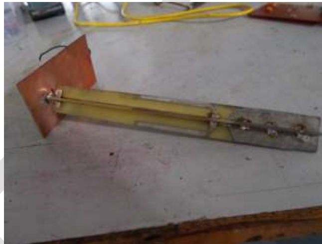
Figure 3 - Antenna mounted circuit
